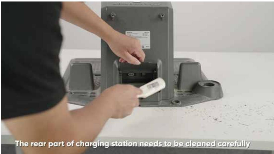
**The rear part of charging station needs to be cleaned carefully**
